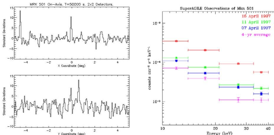
Figure 6. *Left panel:* SA simulated sky images ( $X$  and  $Y$  views) for MKN 501. The AGN is the less intense between the two peaks. *Right panel:* SA simulated spectrum for different emission levels of MKN 501. See Feroci et al. 2002 for more details.
