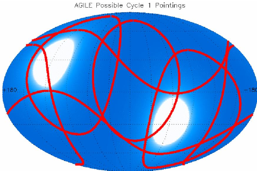
Figure 2. A possible AGILE pointing strategy (AGILE Cycle-1). Red circles are the initial positions of the AGILE-GRID FOV for the six pointings. The blue-scale background represents the Earth occultation factor (for a detailed discussion see Pellizzoni et al. 2001); lighter areas correspond to unocculted sky regions near the Ecliptic Poles. The maximum occultation factor is about 40%.
