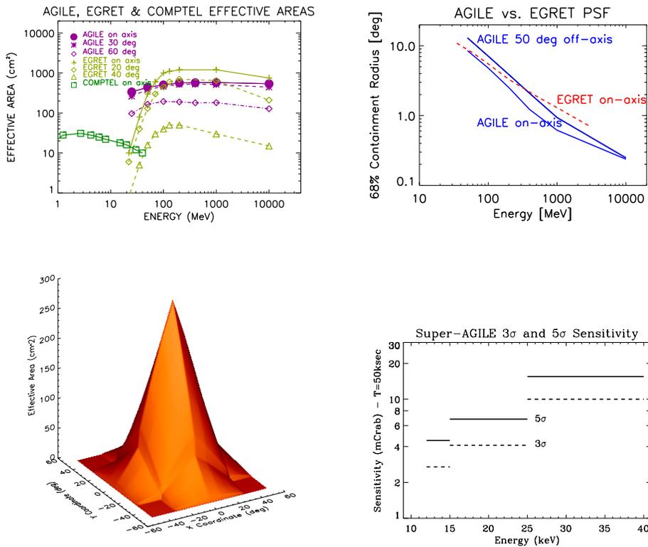
Figure 1. *Top panels:* comparison between the AGILE-GRID and EGRET effective area (left) and angular resolution (right). *Bottom panels:* SA effective area (left) and sensitivity (right).
